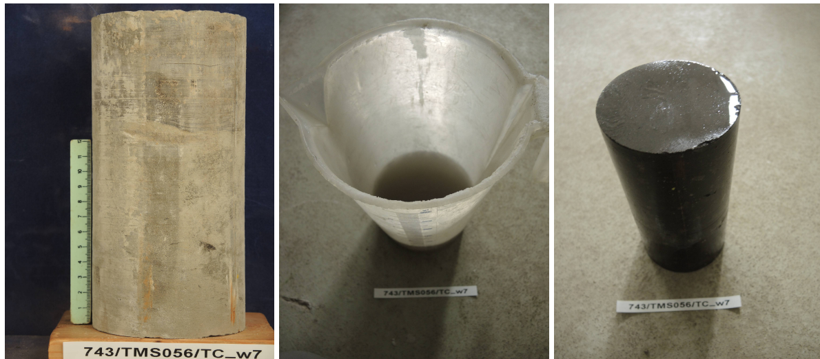
Fig. 3-5: Left: prepared sample under “natural humidity” conditions; Centre: Cylinder in which the samples were totally covered with brine (for 24 h); Right: wet sample after saturation process.
