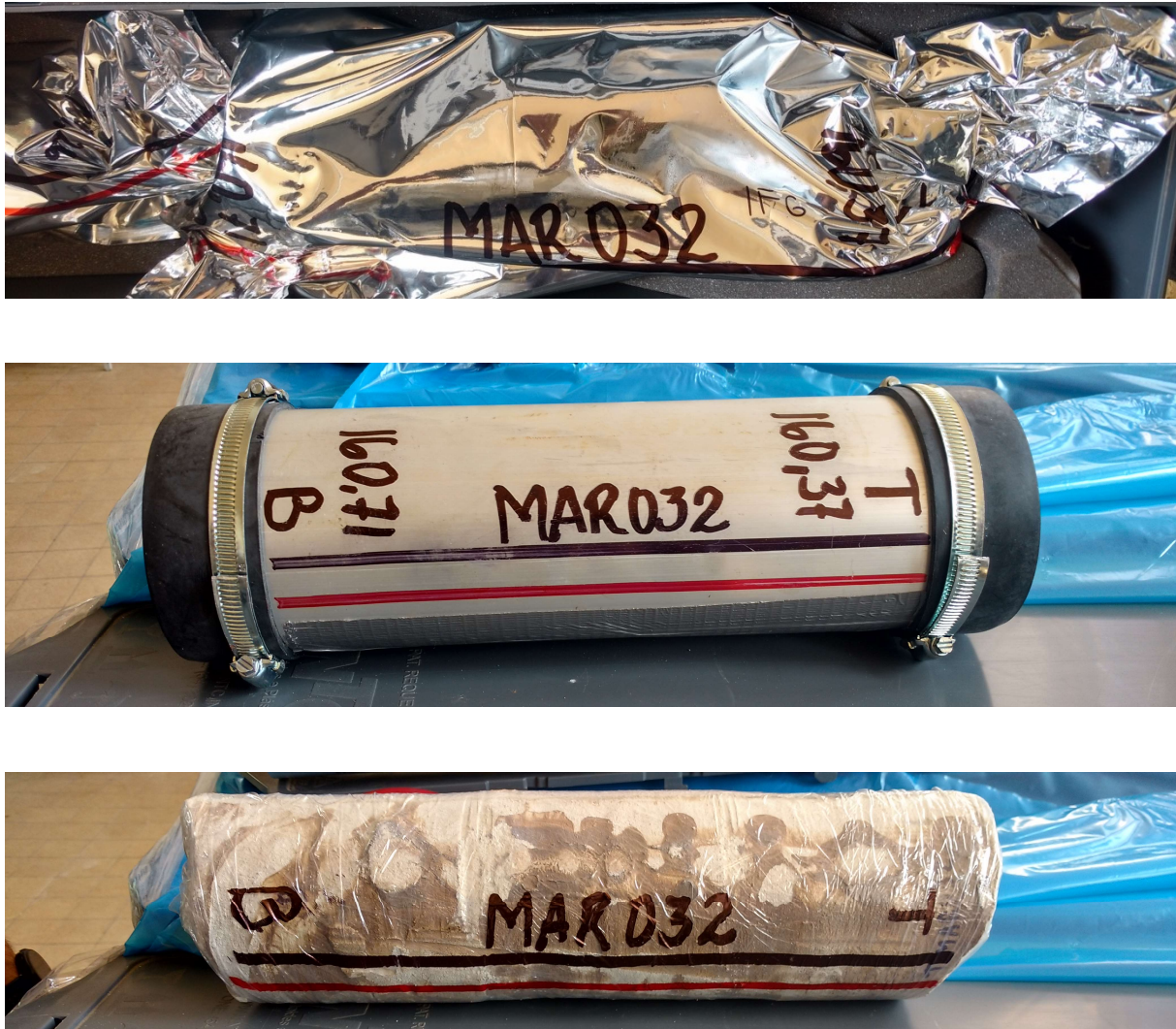
Fig. 2-3: Example of the transport and storage conditions. Top: Core segment covered in aluminium foil; Centre: stable aluminium half-shell container, Bottom: finally, the core segment covered with plastic foil.
