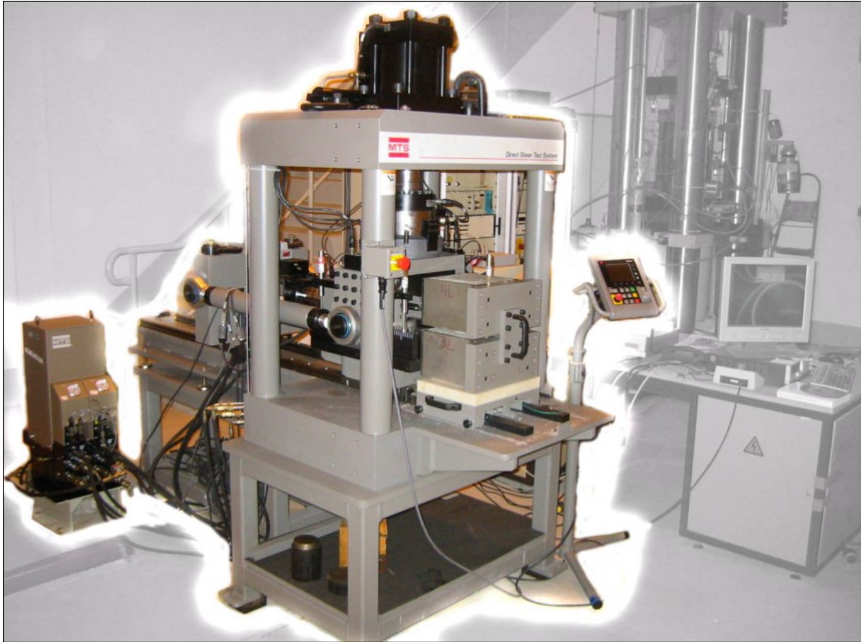
Fig. 3-6: The MTS – shear test system (model 816) for direct shear tests.
